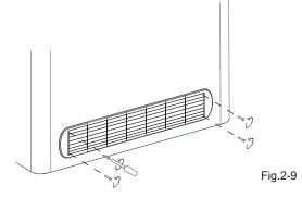
The air filter must be cleaned by blowing it out with compressed air or washing it in water.Before refitting the filter,make sure it is clean and completely dry.If the filter is damaged,it must be replaced with a genuine corresponding filter.
