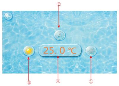
Click the refrigeration mode button (1), automatic mode button(2) or heating mode button (3) then you can select the corresponding mode  $\$ .
