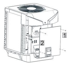
Notes:Touch display installation for magnetic adsorption, can be directly removed
