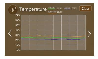
This curve function records the water inlettemperature and water outlet temperature;
