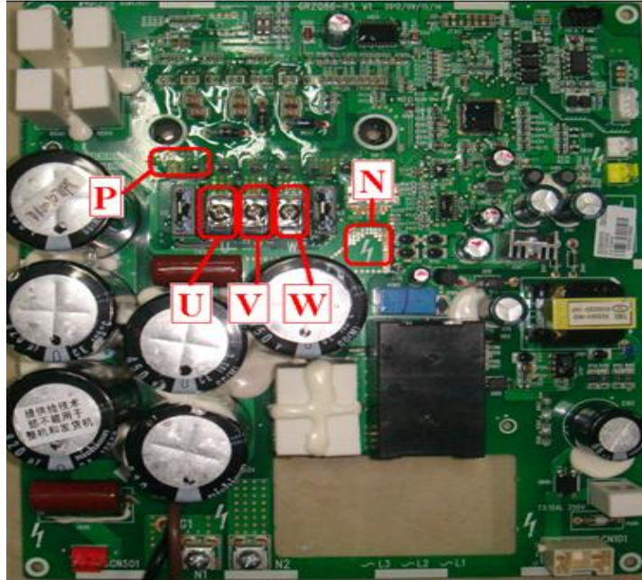
(4) Variable-frequency compressor drive board IPM over-temperature fault (ODU fault P8)
