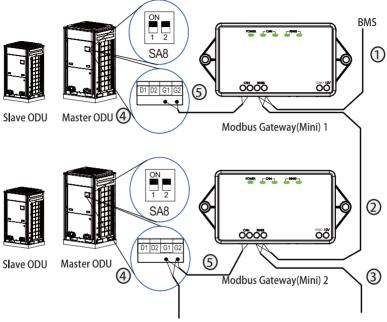
(1) Communication wire connection between Modbus Gateway(Mini) and BMS: Step 1: Confirm the first Modbus Gateway(Mini) (Modbus Gateway(Mini)1 as shown in the figure) that needs to be connected to BMS. Connect the port of RS485 of this gateway and the BMS with communication cable, as shown in step ① in the figure.
