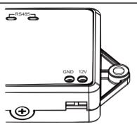
Note: pay attention to the polarity of power input and connect power according to the interface instruction.
