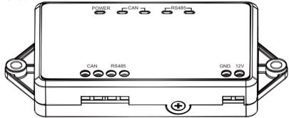
CAN communication interface: It is connected to air conditioner through twocore connection wire, to realize communication between Modbus Gateway(Mini) and air conditioner. RS485 communication interface: It is connected to BMS through two-core communication cable, to realize communication between Modbus Gateway(Mini) and BMS or nearby Modbus Gateway(Mini).
