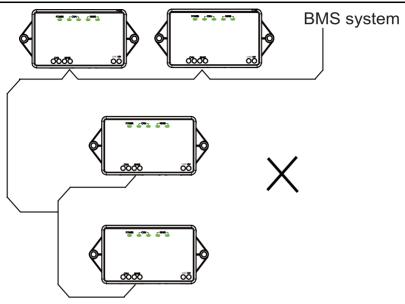
(2) Communication connection between Modbus Gateway(Mini) and air conditioner (n is air conditioner quantity, n≤16);
